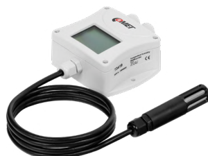
HTemp-485 T3419 Temperature range: -30 to 105 °C, humidity range: 0-100% RH, dew point range: -60 to 80DP °C
